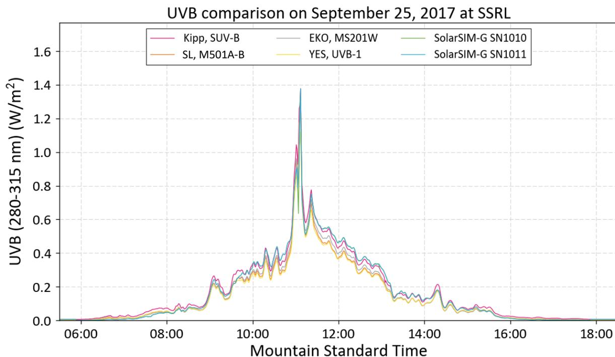
**Figure 9.** UV-B data obtained from the SolarSIM RUs, compared to NREL's M501A-B, SUV-B, MS201W and UVB-1 sensors for the 25<sup>th</sup> September 2017.
