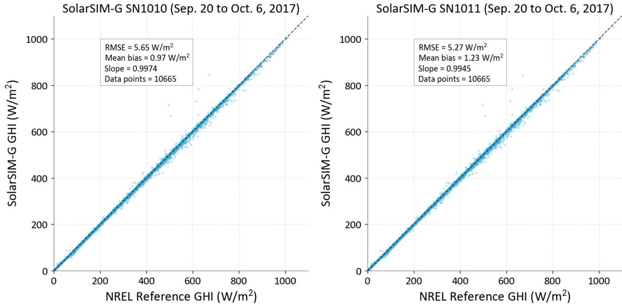
**Figure 13.** Scatter plots of the GHI data obtained from the SolarSIM RUs (SN1010 LHS, SN1011 RHS) plotted against NREL’s reference GHI data for the period 20<sup>th</sup> September to 6<sup>th</sup> October 2017. The RMSEs for both instruments are well within  $\pm 10$  W/m<sup>2</sup> with over 10,000 data points analyzed per SolarSIM.
