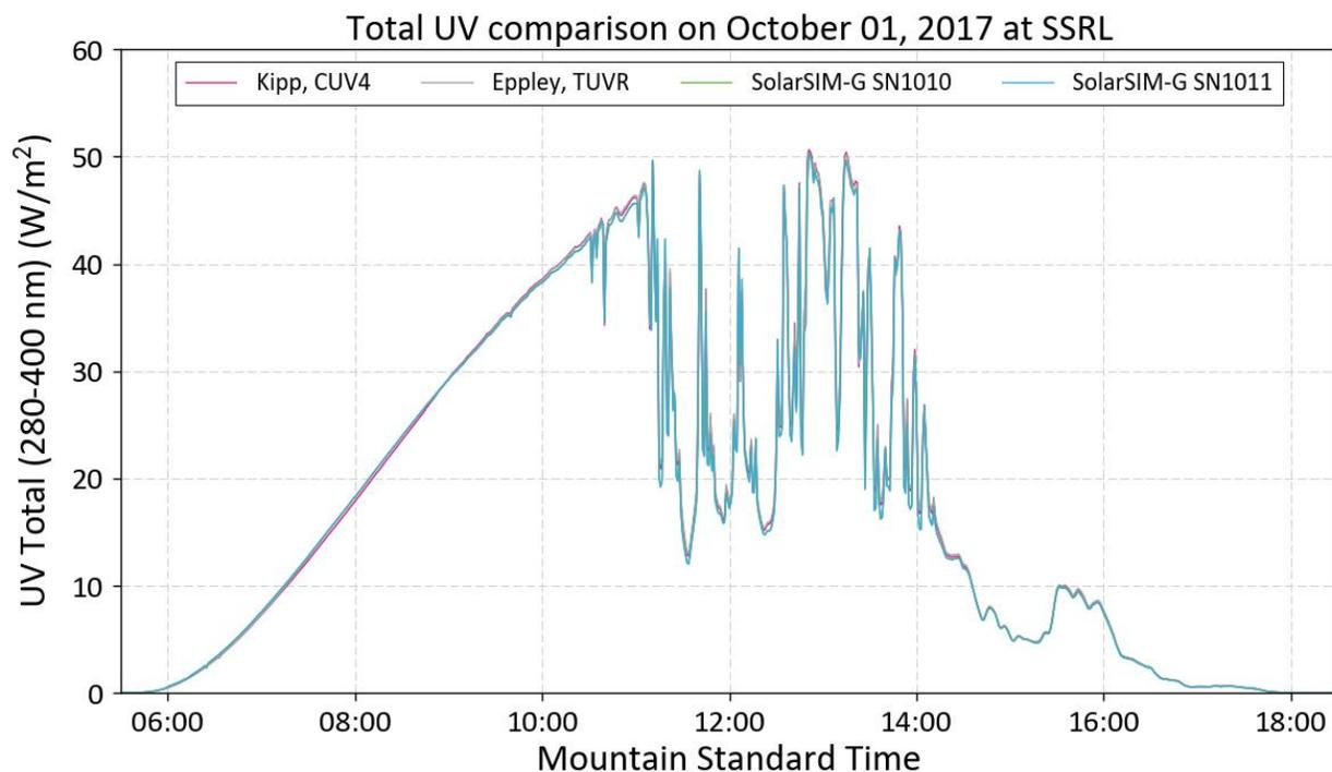
**Figure 5.** UV Total data obtained from the SolarSIM-G RUs, compared to NREL’s CUV4 and TUVR sensors for the 1<sup>st</sup> October 2017.
