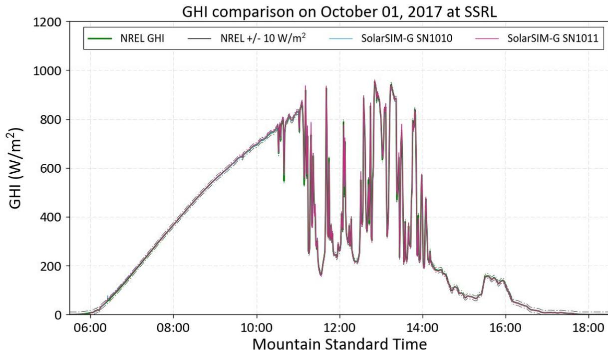
**Figure 11.** GHI data obtained from the SolarSIM RUs, compared to NREL’s reference GHI data for the 1<sup>st</sup> October 2017. The SolarSIM data is consistently within  $\pm 10 \text{ W/m}^2$  of the reference GHI data.
