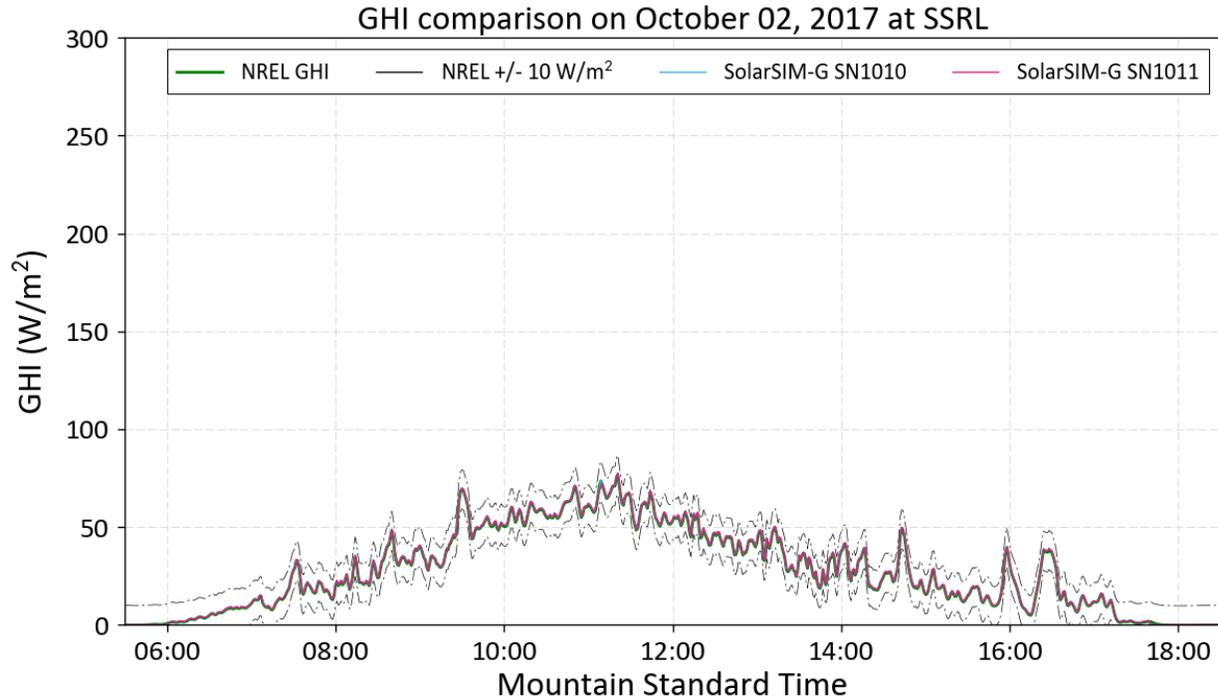
**Figure 12.** GHI data obtained from the SolarSIM RUs, compared to NREL’s reference GHI data for the 2<sup>nd</sup> October 2017. The SolarSIM data is consistently within  $\pm 10 \text{ W/m}^2$  of the reference GHI data.
