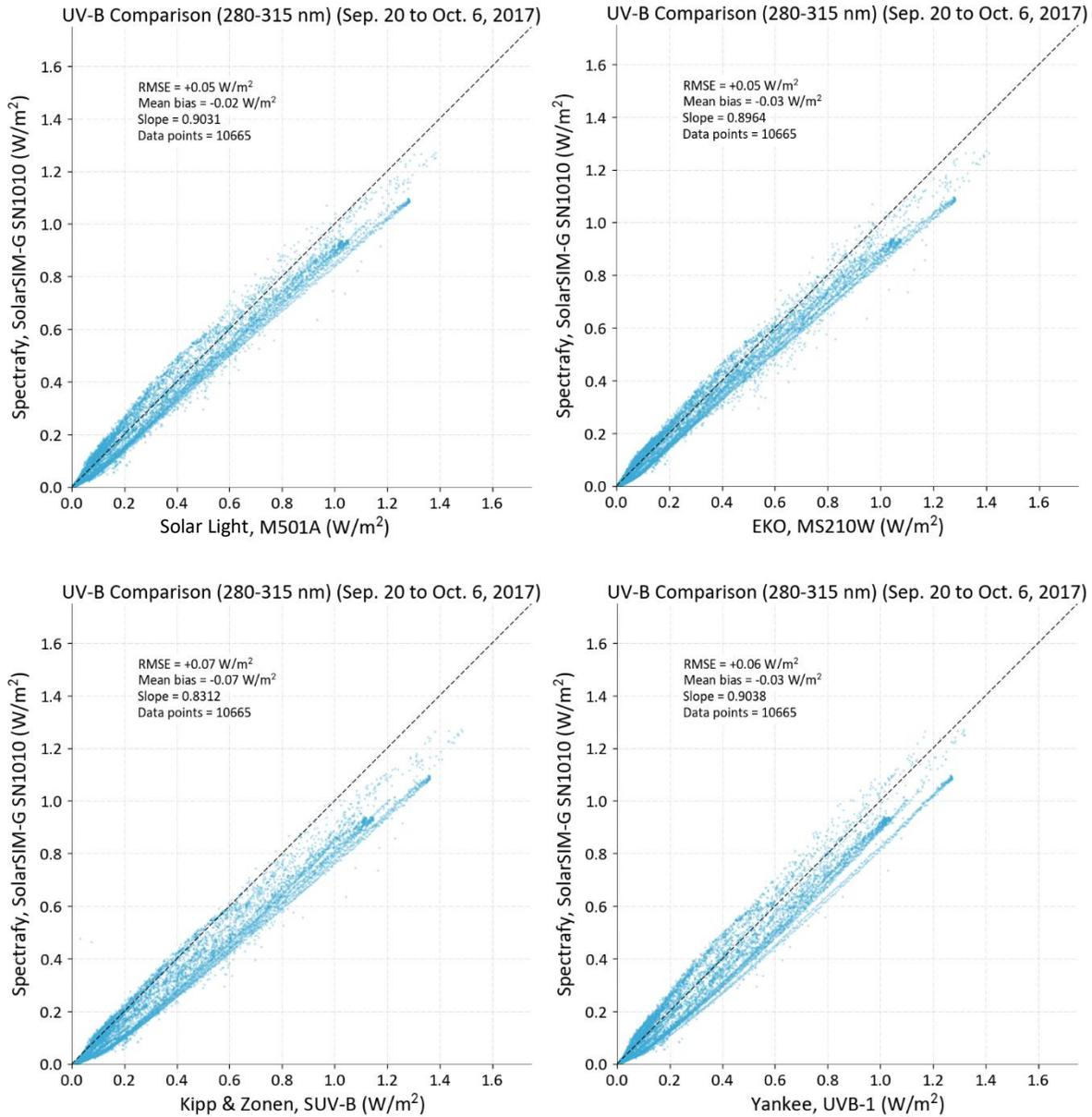
**Figure 10.** Scatter plots of the UV-B data obtained from the SolarSIM RU (SN1010) plotted against NREL's M501A-B (top left), MS210W (top right) SUV-A (bottom left) and UVB-1 (bottom right) for the period 20<sup>th</sup> September to 6<sup>th</sup> October 2017. Over 10,000 data points were analyzed.
