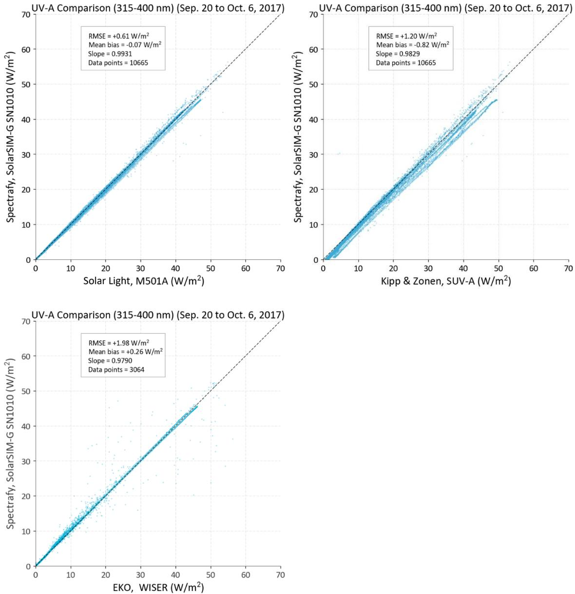
**Figure 8.** Scatter plots of the UV-A data obtained from the SolarSIM RU (SN1010) plotted against NREL’s M501A (top left), SUV-A (top right) and MS711 (bottom left) for the period 20<sup>th</sup> September to 6<sup>th</sup> October 2017. Over 10,000 data points were analyzed. Note that the SUV-A suffered from a non-zero offset during the measurement period.
