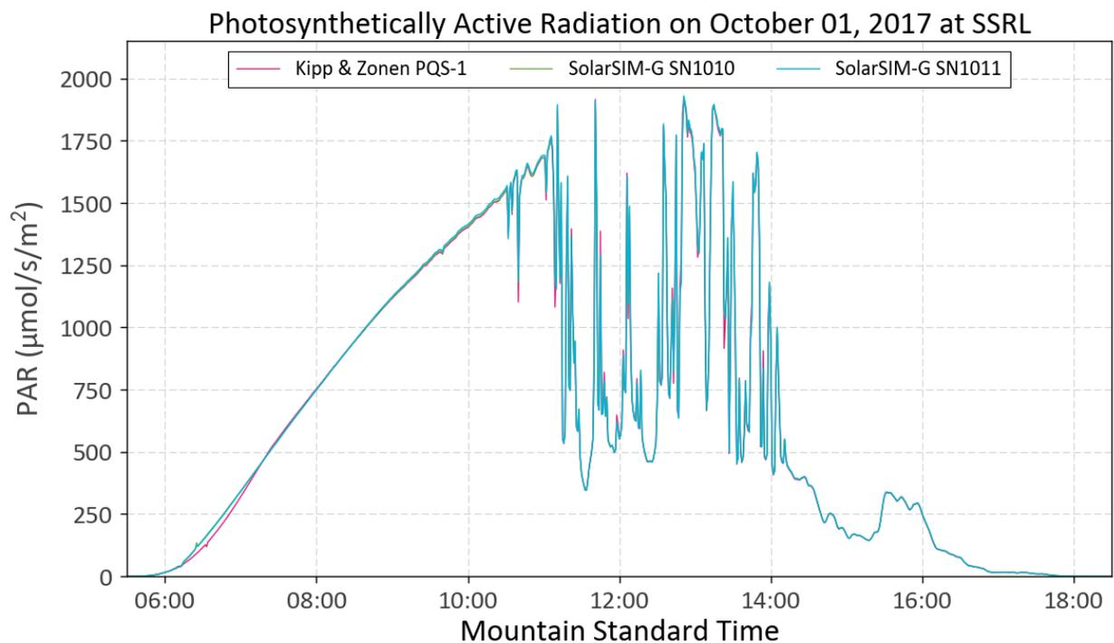
**Figure 9.** PAR data obtained from the SolarSIM RUs, compared to NREL’s PSQ-1 PAR data for the 1<sup>st</sup> October 2017.
