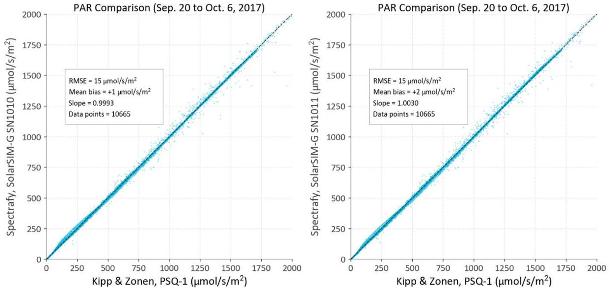
**Figure 10.** Scatter plots of the PAR data obtained from the SolarSIM RUs (SN1010 LHS, SN1011 RHS) plotted against NREL’s PSQ-1 PAR data for the period 20<sup>th</sup> September to 6<sup>th</sup> October 2017. The RMSEs for both instruments are well within  $\pm 15 \mu\text{mol/s/m}^2$  with over 10,000 data points analyzed per SolarSIM.
