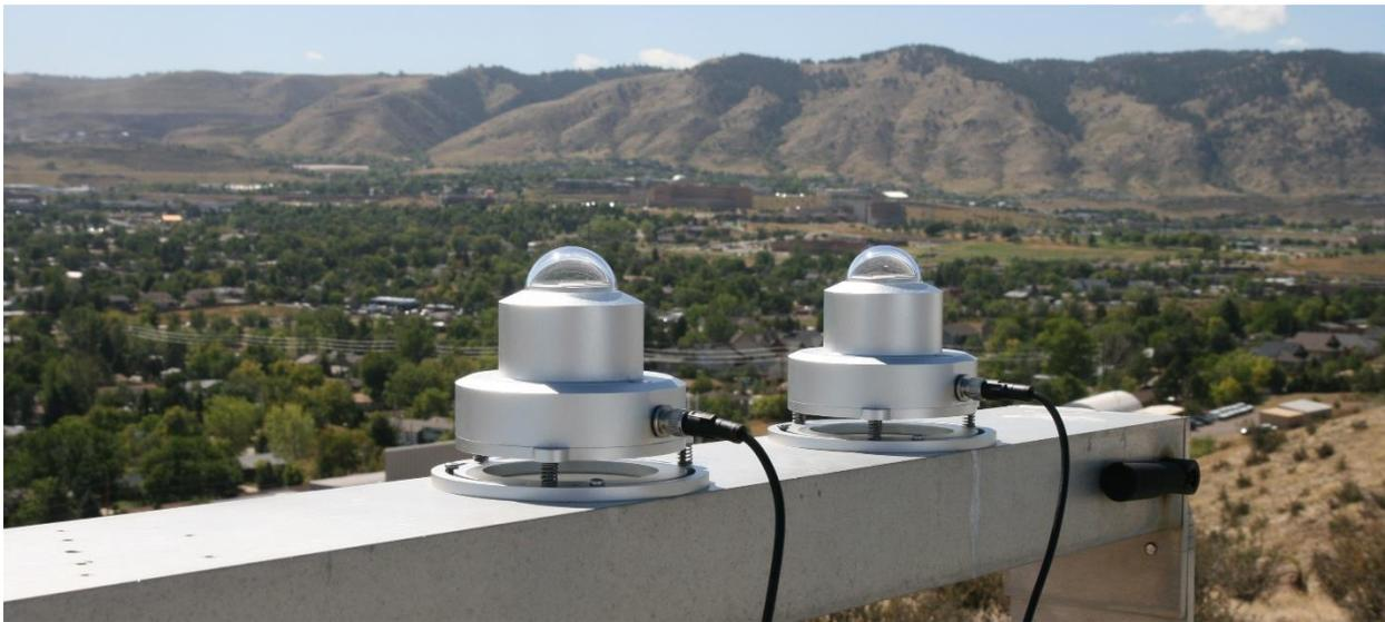
**Figure 2.** The SolarSIM-G/UV reference units in operation at NREL's Solar Radiation Research Laboratory, October 2017.
