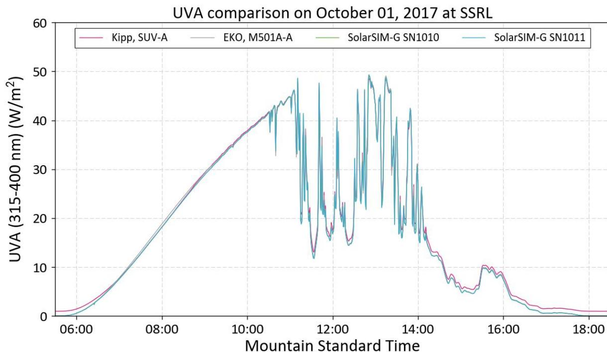
**Figure 7.** UV-A data obtained from the SolarSIM RUs, compared to NREL’s M501A-A and SUV-A sensors for the 1<sup>st</sup> October 2017. Note the zero offset in the SUV-A data.
