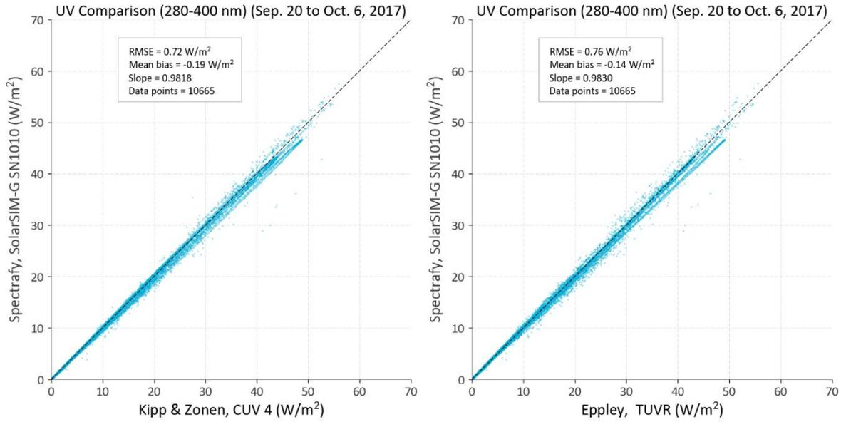
**Figure 6.** Scatter plots of the UV-T data obtained from the SolarSIM RU (SN1010) plotted against NREL's CUV-4 and TUVR UV-T data for the period 20<sup>th</sup> September to 6<sup>th</sup> October 2017. Over 10,000 data points were analyzed.
