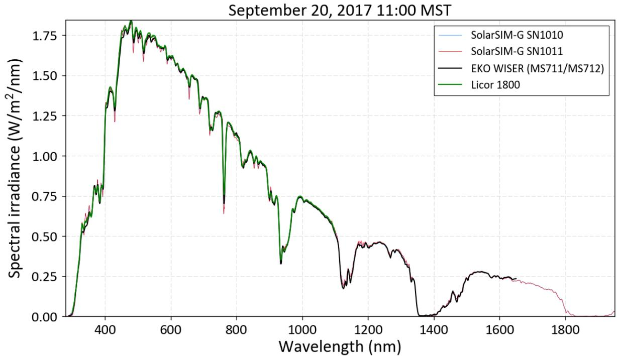
**Figure 4.** Spectral global normal irradiance as measured by the WISER, Licor-1800, and the SolarSIM RUs at 11:00 MST on September 20, 2017. To aid comparison, the spectra obtained from the SolarSIMs have been smoothed with 5 nm central averaging to approximate the lower measurement resolution of the reference spectroradiometers.
