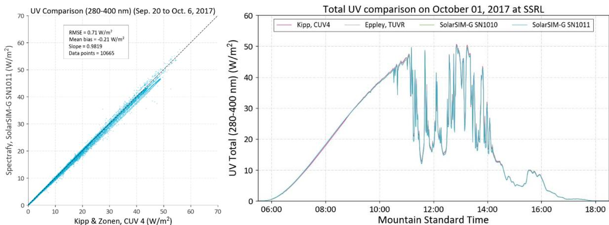
**Figure 1.** Scatter plot of UV-T data obtained from the SolarSIM RUs plotted against NREL reference UV sensors (LHS) and UV-T data obtained from the SolarSIM RUs compared to NREL’s CUV4 and TUVR sensors for 1<sup>st</sup> October 2017.
