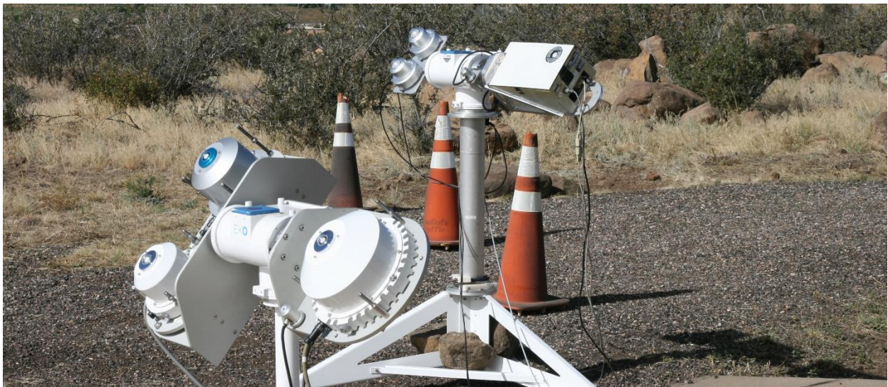
Figure 3. Calibration setup with the SolarSIM-G RUs and Licor 1800 spectroradiometer (background) and the EKO WISER (MS711/MS712) spectroradiometers (foreground).
