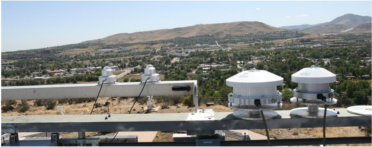
Figure 8. The SolarSIM-G RUs in global horizontal mode on the SRRL deck, alongside NREL's WISER(711/712) spectroradiometers.
