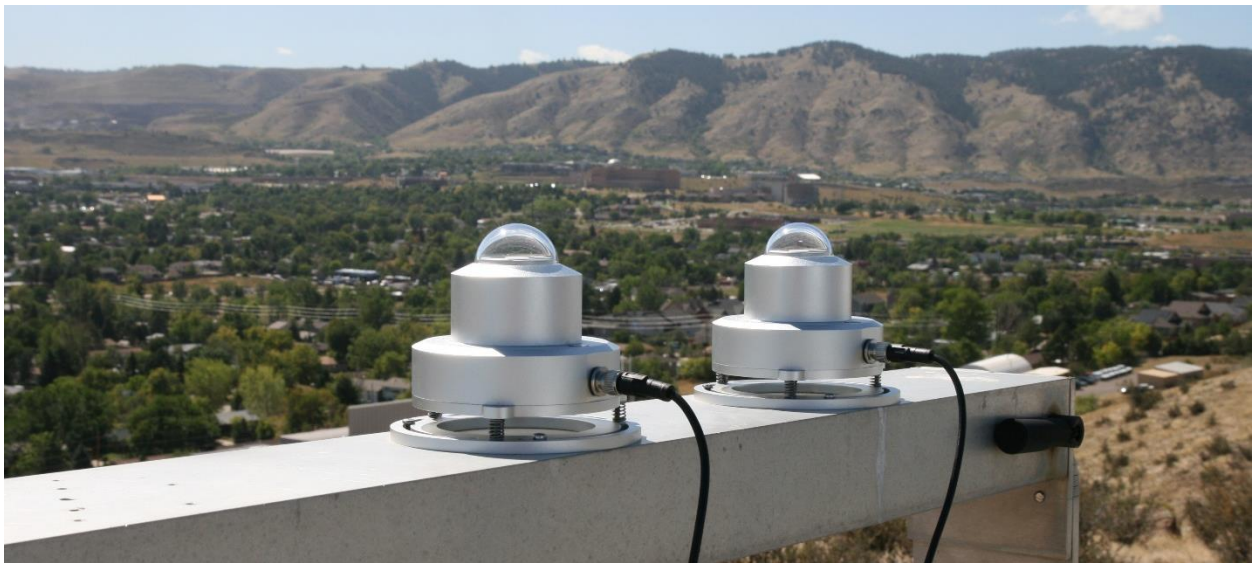
Figure 2. The SolarSIM-G reference units in operation at NREL's Solar Radiation Research Laboratory, October 2017.
